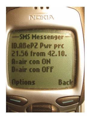
There are two Web Services that deliver this functionality. One of these constantly monitors the electricity prices and provides notification of significant price changes to the customer. The other provides SMS messaging back and forth to the user. Internet-aware controllers and smart meters are used to provide instant and safe control of equipment over the Internet, based on the replies received from the user via SMS.
